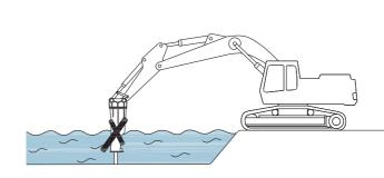
3 Do not allow the breaker to fall to a rock. Falling down the breaker will apply excessive force to the breaker or the carrier, causing damage to the parts of the breaker and carrier.
