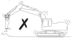
When position is excessive enough to break rocks with front of the base machine raised, the machine may suddenly tilt forward the moment rocks are broken. Then, the breaker body or the end of bracket may violently hit against rocks and result in damage.
