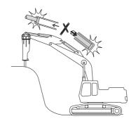
Lifting thing by hanging wire in the bracket or rod not only causes damage to the breaker but also is very dangerous.
