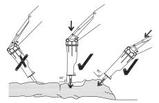
Apply same direction of boom force in line with the rod and place the rod in the rock with hammering surface as vertical as possible. If hammering surface is oblique, the rod may slip during hammering. This causes the rod to seize and to be broken and piston to be damaged. When breaking, fully stabilize the rod first and then select the point of a rock on which hammering can be performed in a stable condition.
