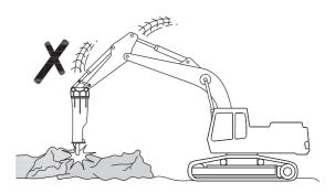
Breaking operation conducted at the stroke end(when the cylinder is extended or retracted to a maximum extent) of respective hydraulic cylinders of the carrier will lead to damage to the cylinders and other parts of the carrier.
