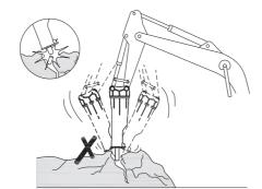
Do not operate breaker when all components except rod are immersed in water and mud. Underwater usage of the breaker will cause internal damage to the breaker.
