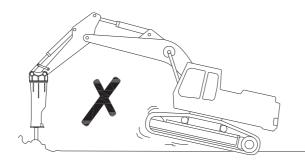
3 It is undesirable to carry out hammering under the below condition, because vibrations during hammering may be transmitted to tracks of the base machine. During hammering, however, proper position must be always applied to the breaker. Special care must be taken not to hammer under abnormal condition.
